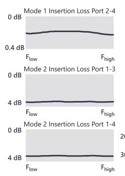
of the configuration shown in the outline drawing on the next page. Please note that the extra waveguide length was provided per customer request. Also, the Mode 2 loss data includes 3 dB loss due to sidewall coupler characteristics.
